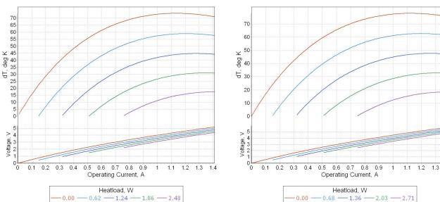
**Note**: Performance data is specified at optimal conditions (TEC hot side is stabilized at ambient temperature). Heatsink thermal resistance is not included into estimations. Use TECCad Software for estimations under different conditions.
